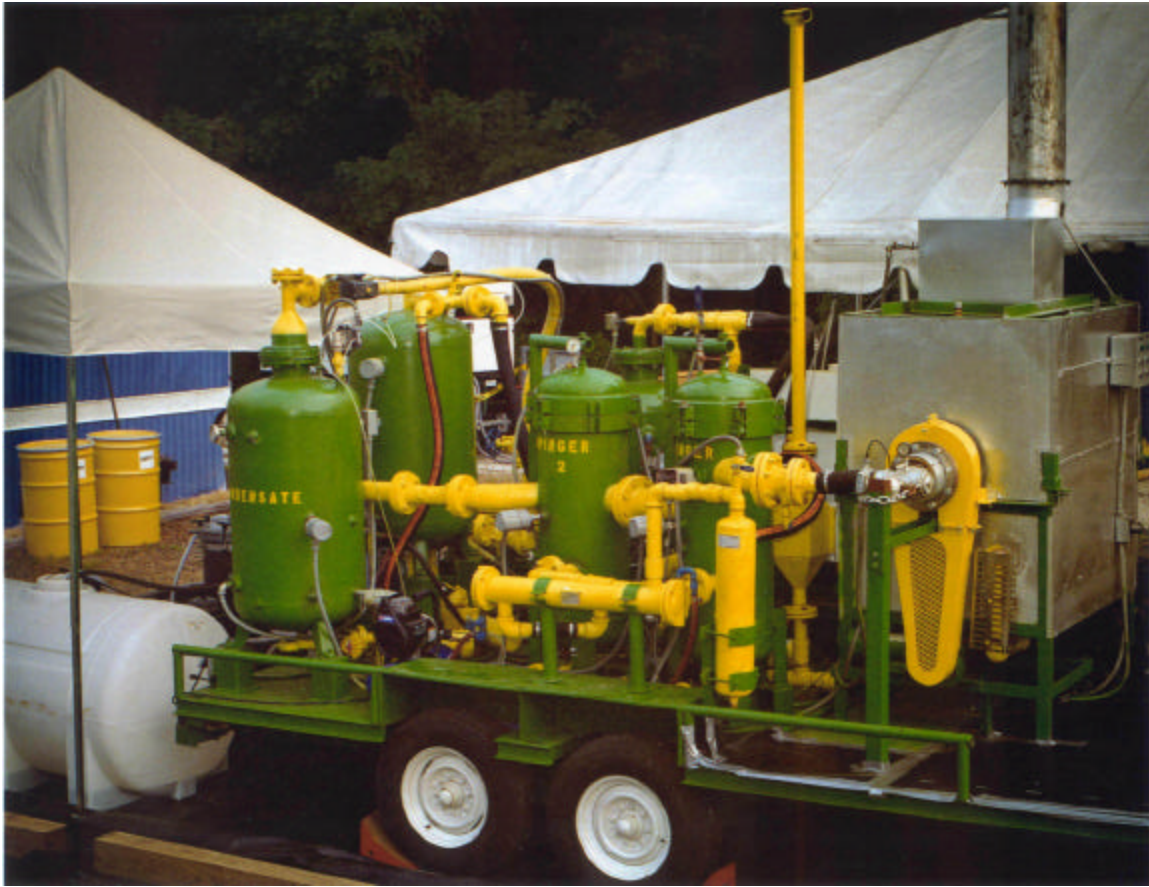
Figure 1. Photograph of the SepraDyne™-Raduce trailer mounted rotary retort system.
